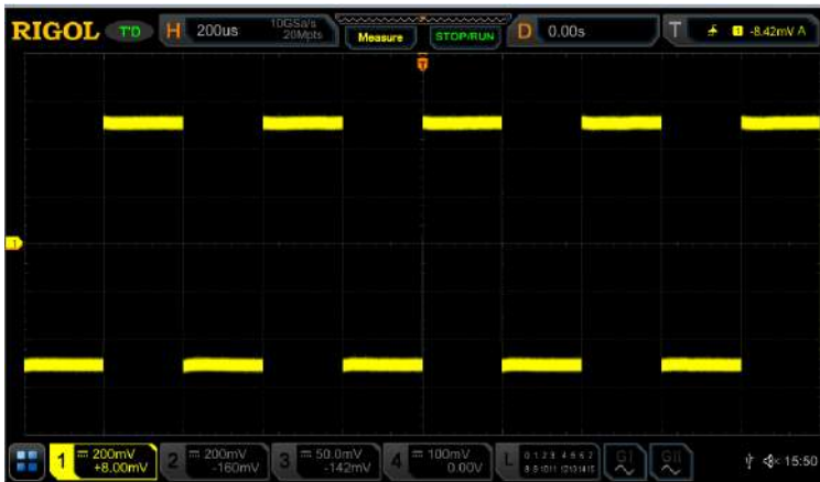
Figure 4-2 Waveforms before Averaging
