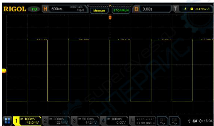
Figure 4-3 Waveforms after 128 Times of Averaging
